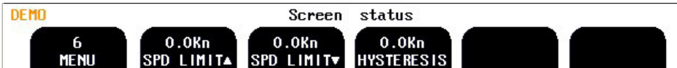
Screen status, Menu 6, speed limits and hysteresis
